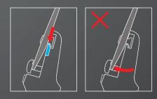
After release, the impact from the string is directed vertically from the limb's contact point of the riser block. Super engineered plastic with excellent mechanical properties of the block adds resistance to heat, shock, along with wear and tear.
